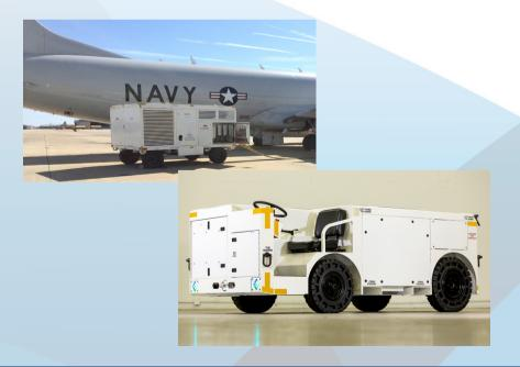
Few environments are more challenging for ground support equipment than the flight deck of an aircraft carrier. JBT has been contracted to provide self-propelled power carts, capable of delivering 28VDC, 270VDC, and 400 Hz AC power to carrier-based aircraft. JBT also supplies 45 ton, diesel powered conditioned air carts for shore-based naval aircraft.
